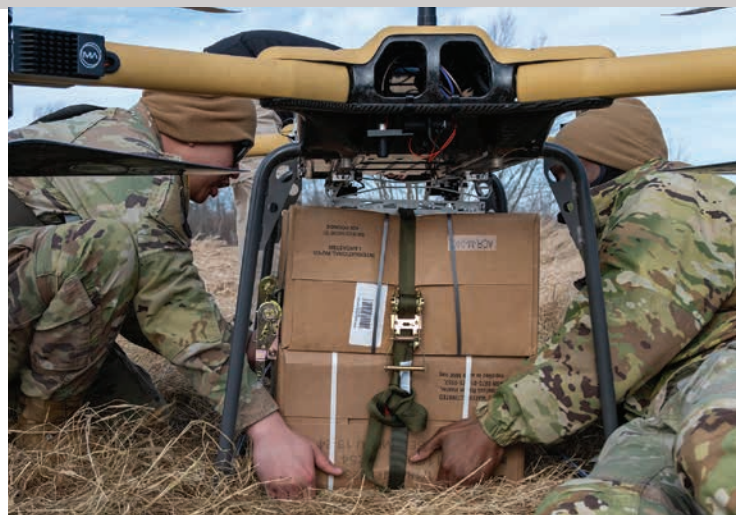
The 10th Mountain Division continues to test medium and heavy quadcopter tactical resupply vehicles (TRV), such as the TRV-150, denoting that it can carry up to a 150lb payload. A single TRV-150 can deliver emergency resupply of batteries or ammunition. If flown as a group, multiple TRV-150s could simultaneously refit a platoon in one lift. (U.S. Army photo by Sgt. First Class Neysa Canfield)
